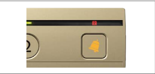
Emergency Operation mode lamp on Car Operating Panel will blink.
